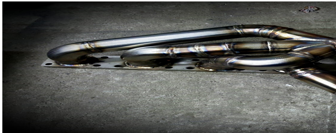
singlescrol options -&gt; wastegate pipe FRONT
